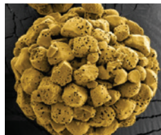
SEM (scanning electron microscope) image illustrates the morphology of N-ZORBIT™ 2144 DG plating agent's agglomerated microporous starch granules.
